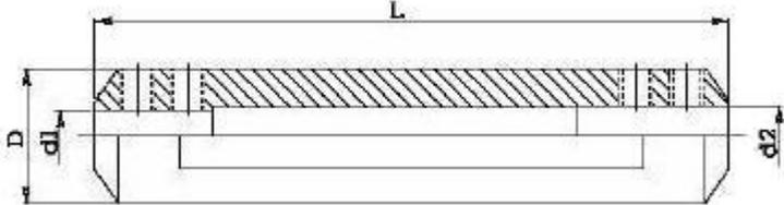
The technical drawing shows a side view of a double boring bar sleeve. It is a long, cylindrical component with a central hole. The outer diameter is labeled 'D', the inner diameter of the central hole is labeled 'd1', and the diameter of the outer hole is labeled 'd2'. The total length of the component is labeled 'L'. The drawing includes hatching to indicate the internal structure and the location of the two holes.
